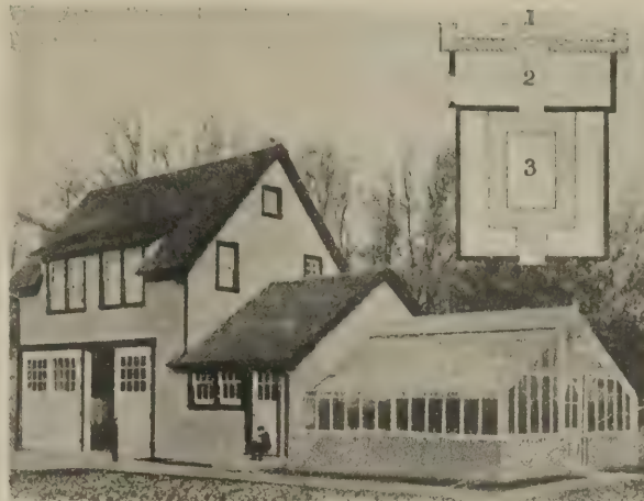
Greenhouse in combination with garage, separated by workroom. This simplifies heating and is an economical and popular form
